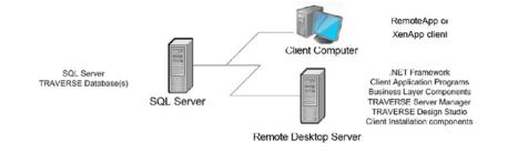
Figure 2 - Ultra thin-client Traverse installation example (Microsoft RDS or Citrix XenApp)
